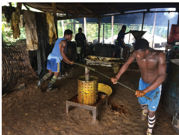
Figure 6. Workers operating a hand-press for palm oil extraction, commonly used in small-scale processing systems, achieve lower oil extraction efficiency than large-scale mills.
