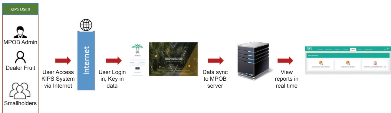
Figure 4. The operational flow of the KIPS system.
